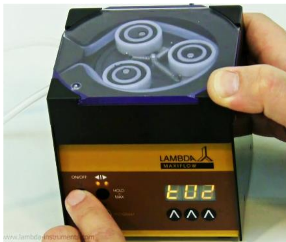
Figure 2-12 Press the ON/OFF button again, the symbol “t02” will briefly appear on the display.
