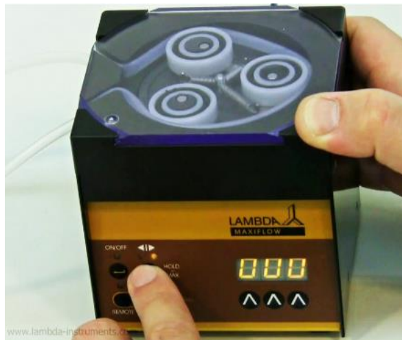
Figure 2-10 Select the direction of the pump rotation using the direction button ◀▶ for each flow rate program.
