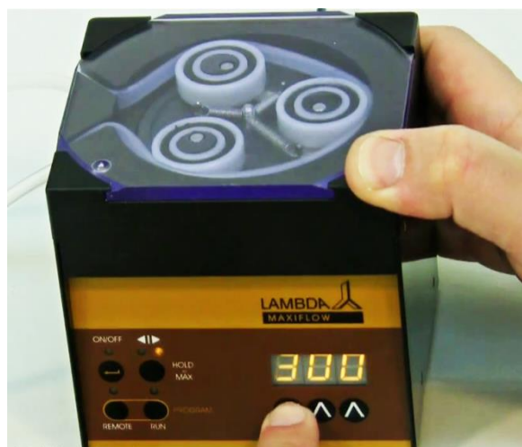
Figure 1-11 The ▲▲▲ buttons can be used to set the desired flow rate.
