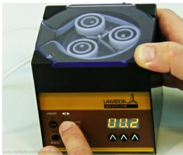
Figure 2-14 Press ◀▶ button, to set the time resolution.
