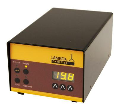
OXYMETER measures the concentration of the  $O_2$  in outgas/exit gas.
