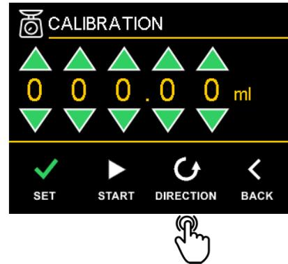
2. After preparation of the measuring device, start the calibration (pumping) by clicking on the "**START**" icon.
