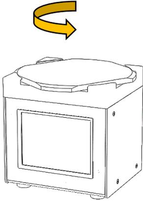
Gently press on the cover glass and rotate it counter-clockwise.
