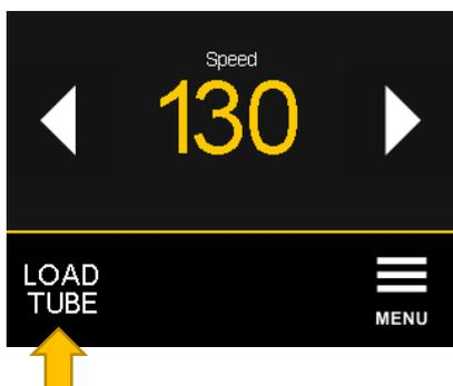
3. Test the selected speed before insertion of tubing into LAMBDA PRECIFLOW *touch*, HiFLOW *touch* or MAXIFLOW *touch*. For LAMBDA MEGAFLOW *touch*, employ the lowest speed when inserting the tubing.
