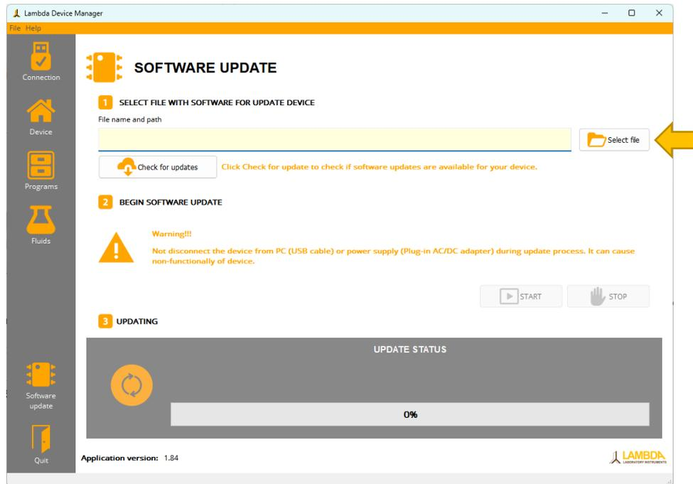
7. Click the **“Select file”** button and browse the path to the decompressed peristaltic pump software file (**pump-2-X.YY.hex**).
