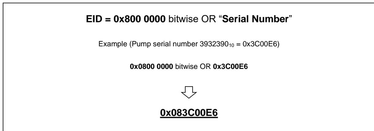
If you use, for example, a 32-bit integer to compose the EID, you need to clean it up using bitwise AND 0x1FFFFFFF.
