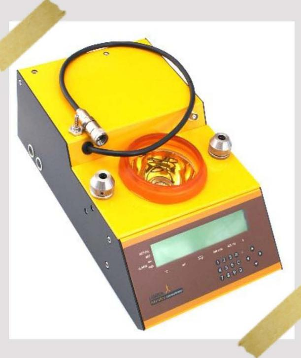
Minimum bioreactor foot print - comparable to the size of an A4 sheet of paper (220 x 400 mm)
