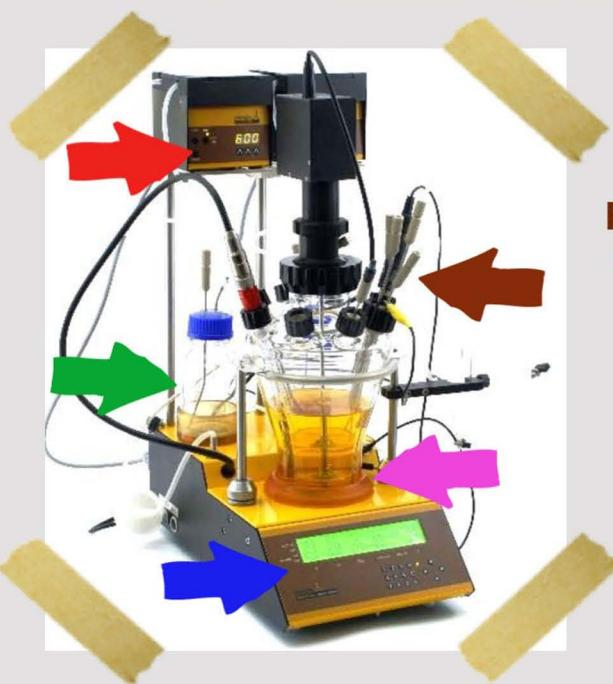
Easily accessible connections: Probes and ports are at an angle of 30° for easy ergonomic handling
