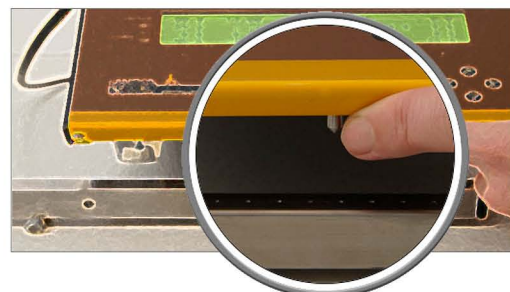
Miniature scale module (steel tip) placed under MINIFOR for easy weight control
