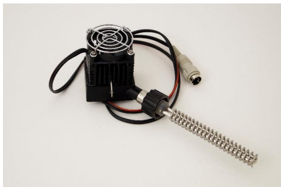
Figure 4-1 Peltier electro-thermal cell, which generates cold (no water cooling system is therefore necessary). The temperature of the cool side is electronically controlled to about +4°C. This prevents freezing of condensed water and blocking of the air way. A small LED on the front of Peltier unit shows when the current is switched on and off. The cable of Peltier cell is connected to the corresponding socket on the rear of the AeroSilento air compressor.
