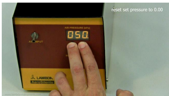
Figure 1-5 When both buttons ▼ and ▲ are pressed simultaneously, the compressor is reset to 0 kPa.
