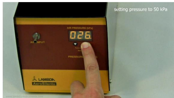
Figure 1-4 Press the ▼ and ▲ buttons once again to set the desired pressure in kPa. The speed of the compressor motor will automatically be adjusted to the required flow rate until the pre-set pressure is attained.
