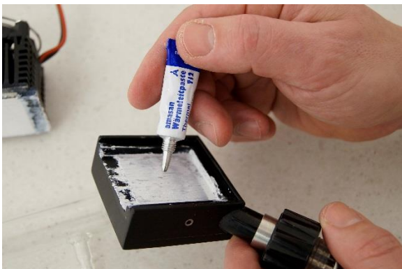
Figure 4-5 Apply the heat-conductive paste on the white surface of the Peltier cooling element with control electronics and fan, before attaching the condensing finger with the unit. Spread out the heat-conductive paste on the surface evenly and thinly ensuring that there are no trapped air bubbles.
