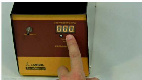
Figure 1-3 Press the ▼ or ▲ button once, to see the preset pressure value. A point is displayed on the last digit.
