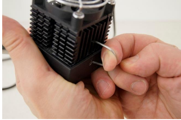
Figure 4-8 Locking clamp has to be pulled firmly through the Peltier cooling element with control electronics and fan and fixed into the hole on both sides of the cell, to make the Peltier cooling finger intact.
