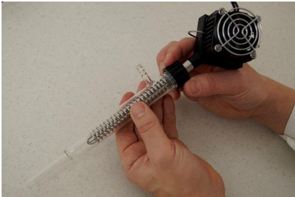
Figure 4-9 Insert the condenser cylinder with the tubing connection over the condensing finger and tighten it securely by the black screw cap.
