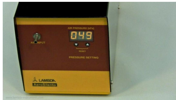
Figure 1-2 Switch the power on with mains switch at the rear of the air compressor. The display indicates the actual pressure.
