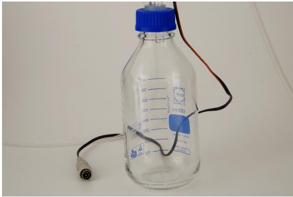
Figure 4-3 Condensate bottle, which is made of pressure resistant chemical glass. The stopper carrying air input and lower part of condenser input tube is screwed to the condensate bottle. The condensate bottle must be protected from shocks and must be kept in the protective stand.
