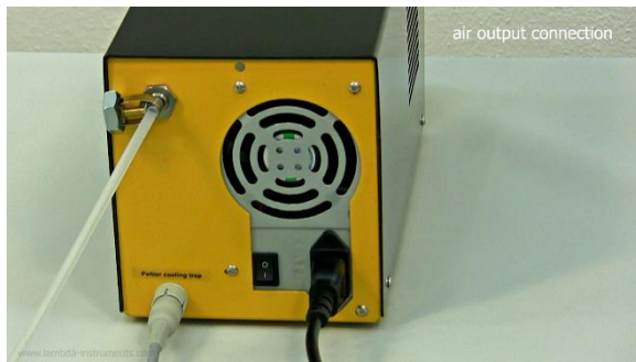
Figure 1-1 Connect the tubing to the air output hose barb on the rear of the AeroSilento and to the tubing barb of the instrument or recipient to be supplied with the compressed air (e.g. to the air input hose barb on the back of the LAMBDA MINIFOR laboratory fermentor-bioreactor).
