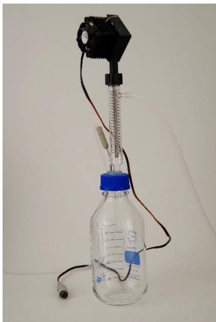
Figure 4-10 Fix the condenser cylinder with the Peltier cooling finger to the condensate bottle.
