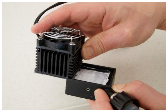
Figure 4-6 Attach the Peltier cooling element with control electronics and fan with the condensing finger, by placing the white surface with the thermal paste onto the respective trap in the condensing finger attachment as shown.
