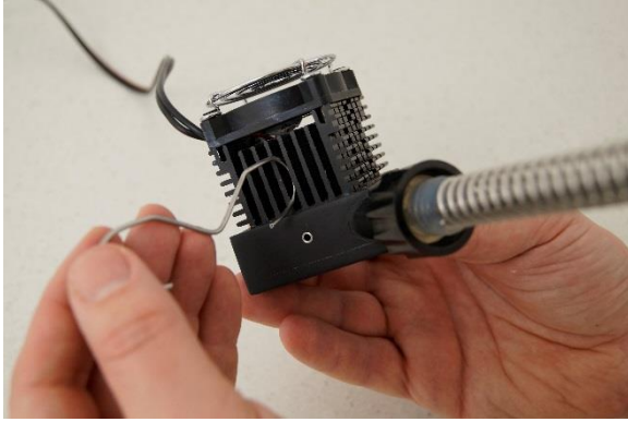
Figure 4-7 The attached peltier cell with the condensing finger should be made kept together with the help of the locking clamp.
