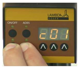
**Figure 2-13:** Press both **REMOTE and RUN** buttons simultaneously and the indication "c01" will appear on the display.
