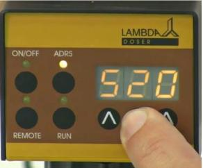
**Figure 2-8:** Enter the desired flow rate for the second program step.
