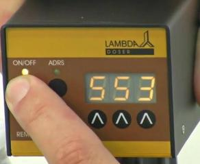
**Figure 1-13:** Choosing the speed of powder addition with the help of control buttons  $\Lambda \Lambda \Lambda$ .
