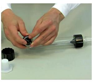
**Figure 1-6:** Place the teflon treated rubber seal on the centering part with the teflon layer facing outside (towards the glass vessel).
