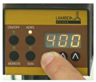
**Figure 2-4:** Set the desired flow rate value for the first program step by pressing the buttons ΛΛΛ below the display (from 0 to 999, corresponding to 0 to 100% of the motor rotation speed).
