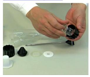
**Figure 1-1:** Insert the ground glass piece through the threaded screw cap SVL 42.
