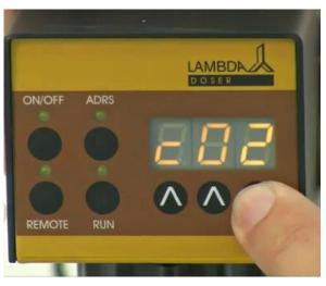
**Figure 2-14:** If the same program has to be repeated twice, increase the cycle number to "c02" by pressing the buttons  $\Lambda$   $\Lambda$   $\Lambda$  below the display (from 0 to 99 cycles).
