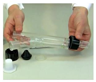
**Figure 1-3:** Screw and secure the ~0.2 I glass vessel to the screw cap with the teflon disc and ground glass piece.
