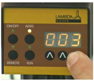
**Figure 2-6:** Select the desired time period for the first program step by pressing the buttons **ΛΛΛ** below the display (from 0 to 999 minutes or 00.0 to 99.9 minutes).
