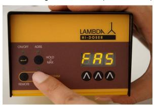
**Figure 1-15** Plug-in the power supply and at the same time press the **RUN** button on the control panel. The display will show the last used mode (**FAS** / **SLO**).
