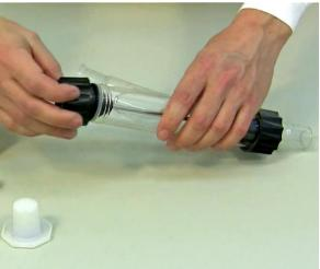
**Figure 1-8:** Secure the centering part with the rubber seal through the axis of the distributor with the screw cap to the glass vessel.
