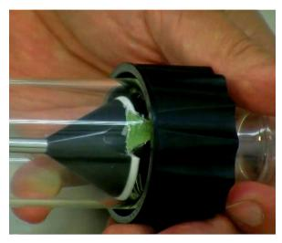
**Figure 1-5:** A silicon baffle/scrapper can be found on the lowest part of the glass vessel. The distributor must be turned with its opening towards the baffle/scrapper.
