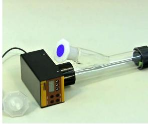
**Figure 1-12:** The solid is added through the filling side arm of the glass vessel. The filling side arm can be closed with a ground glass or plastic stopper.
