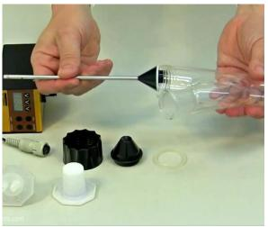
**Figure 1-4:** Insert the distributor (standard) inside the ~0.2 I glass vessel with its opening directed downwards so that it will not be damaged.
