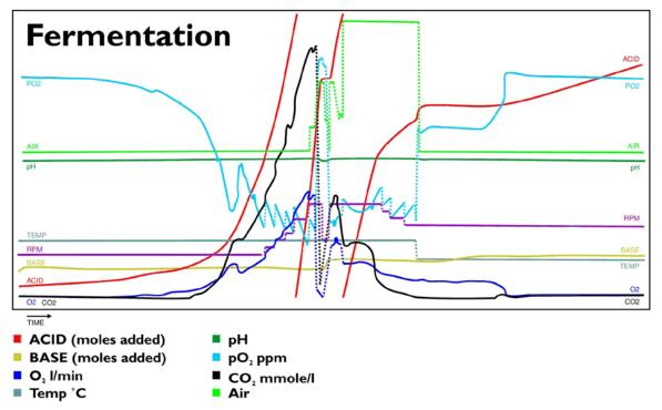
Addition of acid or base necessary to keep the pH constant would not appear without PRECIFLOW and integrator
