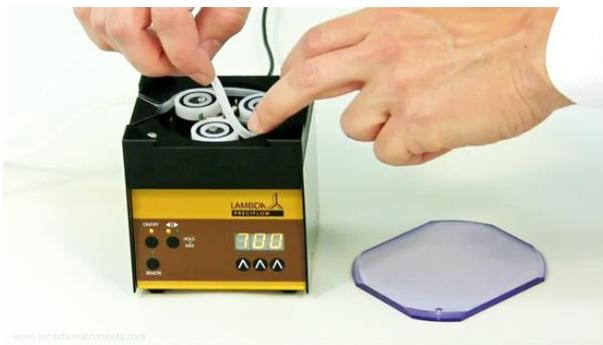
**Figure 1-7** Guide the tubing in the sense of rotation around the slowly turning plastic bearings towards the front slot (on the pump head).
