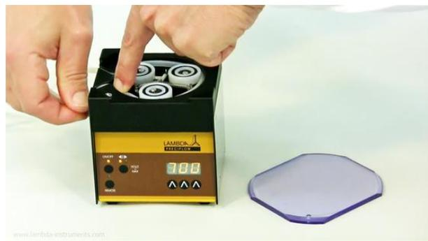
**Figure 1-8** Press the tubing into the front slot on the pump head to secure it in place.
