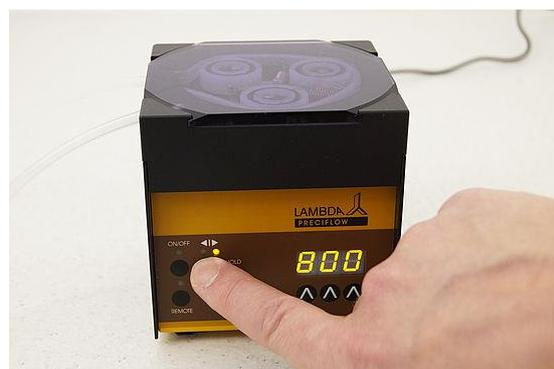
**Figure 1-16** LED illumination in the direction  $\blacktriangleright$  indicates the anticlockwise rotation.
