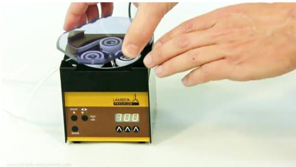
**Figure 1-9** Place the transparent cover back on the peristaltic pump head.
