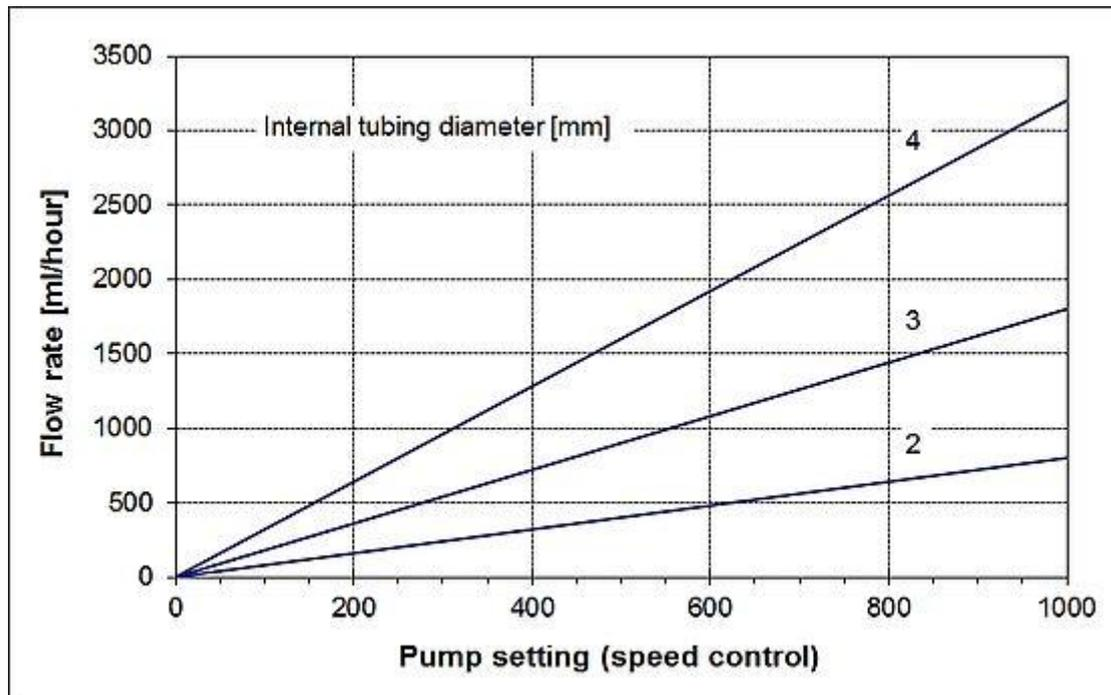
Figure 8-3 Flow diagram of the LAMBDA HiFLOW peristaltic pump when using silicone tubing with inner diameters of 2 mm, 3 mm, 4 mm
