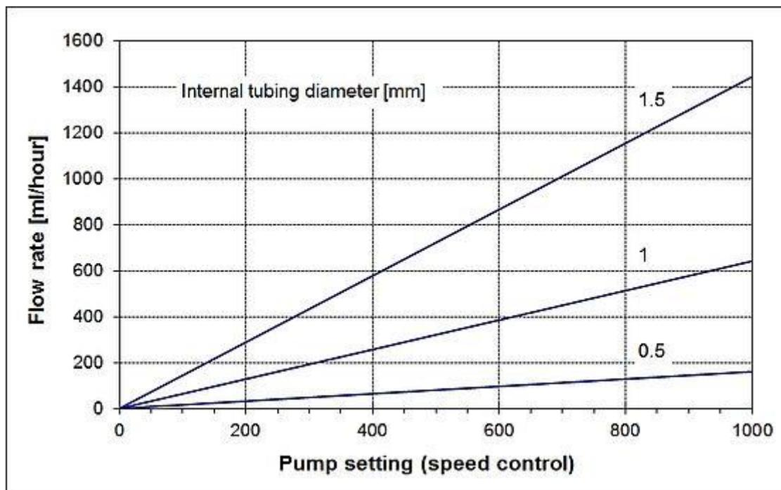
Figure 8-6 Flow diagram of the LAMBDA MAXIFLOW peristaltic pump when using silicone tubing with inner diameter of 1.5 mm, 1.0 mm, 0.5 mm
