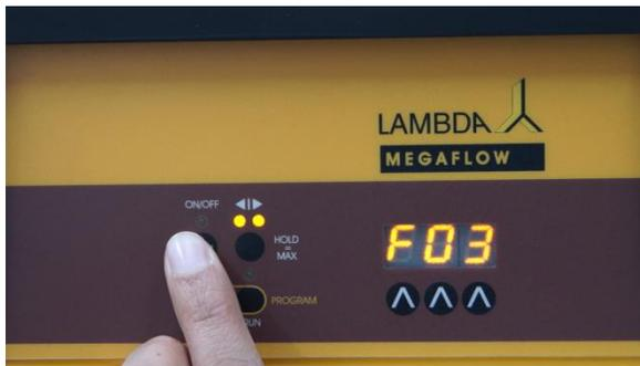
**Figure 2-15** After having entered the time of the last program step, press the **ON/OFF** button.
