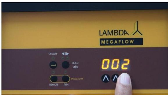
**Figure 2-7** Select the desired time period for the first program step by pressing the buttons  $\wedge \wedge \wedge$  below the display (from 0 to 999 minutes or 00.0 to 99.9 minutes).
