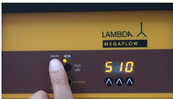
**Figure 2-11** If the  $\triangleleft \triangleright$  button is not used to change the flow direction (clockwise/counter-clockwise), default pump rotation for the set speed is clockwise,  $\triangleleft$  LED ON.
