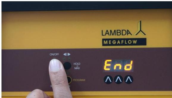
**Figure 2-19** Press the **ON/OFF** button until the indication “End” appears on the peristaltic pump display to confirm and save the program
