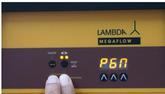
**Figure 2-1** Simultaneously press the **REMOTE** and **RUN** until indication “PGM” appears.
