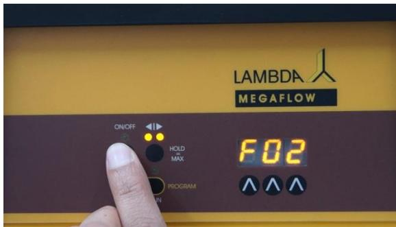
**Figure 2-9** Press the **ON/OFF** button. The indication “F02” will briefly appear on the display indicating that the flow rate (speed) of the second program can be entered.
