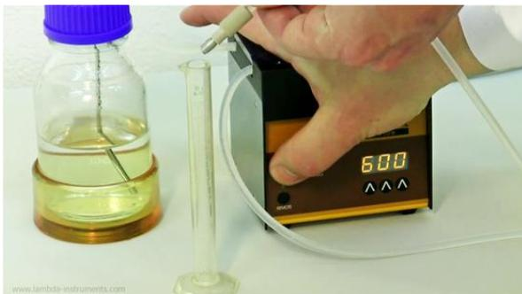
**Figure 3-1** Turn ON the pump and collect the pumped liquid for a measured time (60 seconds) in a graduated cylinder.
