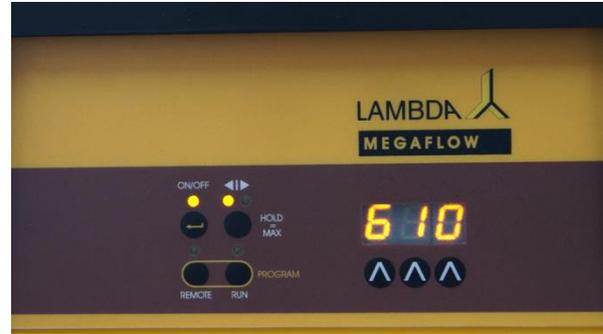
**Figure 1-12** The peristaltic pump will run with the last set speed and flow direction setting.
