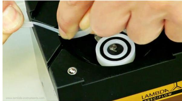
**Figure 1-6** Press the tubing into the back slot on the top of the peristaltic pump. Thin tubing should be pushed completely to the bottom.
