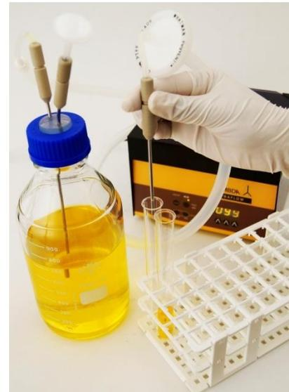
**Figure 9-1** LAMBDA MEGAFLOW with foot-switch for sterile dosing of liquid media in microbiology
