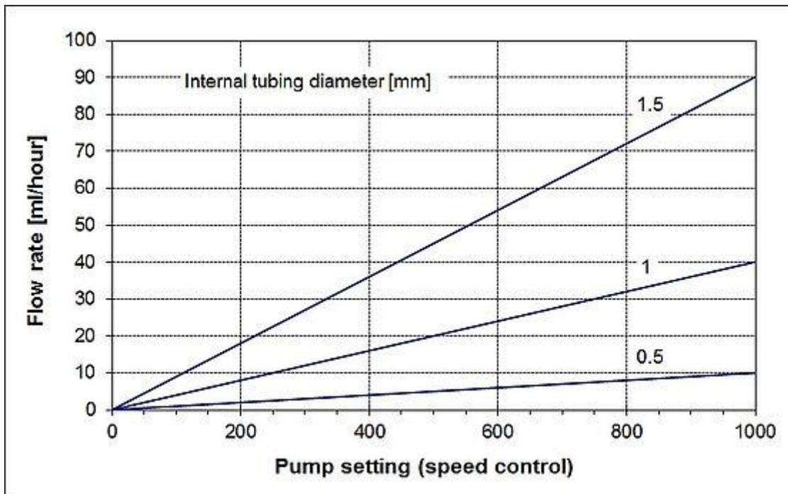
Figure 8-2 PRECIFLOW & MULTIFLOW flow diagram for silicone tubing with inner diameter of 1.5 mm, 1.0 mm, 0.5 mm
