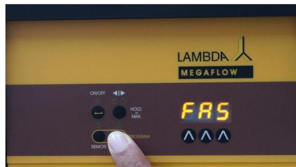
**Figure 1-18** The display shows the default mode **FAS** or the last used mode (**FAS / SLO.**).
