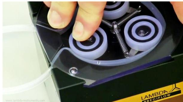
**Figure 1-10** Turn the cover so that the steel ball embedded in the left-front corner of the peristaltic pump fits into the notch in the cover.
