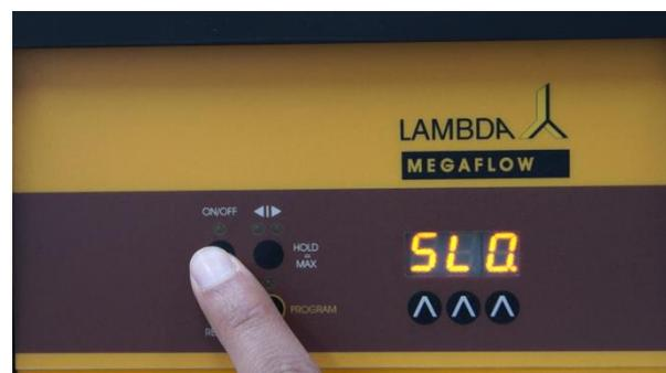
**Figure 1-20** Confirm and save the chosen speed mode by pressing the **ON/OFF** button on the MEGAFLOW pump.
