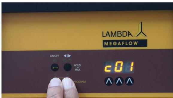
**Figure 2-17** Press the **Remote** and **Run** button simultaneously. The indication “c01” appears on the display. “c01” indicates that the program is executed only once and the peristaltic pump then stops.
