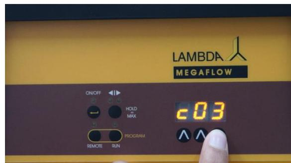
**Figure 2-18** If you wish to repeat the same program 3 times, increase the cycle number to “c03” by pressing the buttons  $\wedge \wedge \wedge$  below the display.
