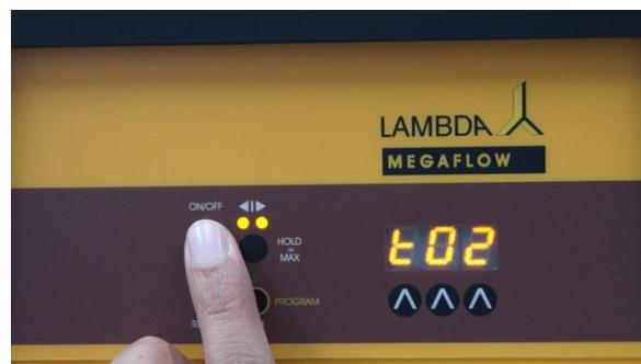
**Figure 2-12** Press the **ON/OFF** button again, the indication “t02” will briefly appear on the display.
