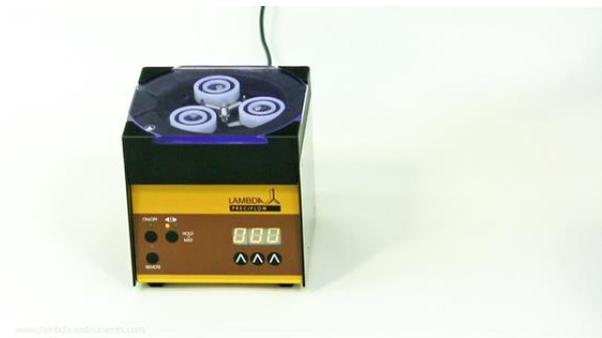
**Figure 1-2** Plug the power supply into the AC mains (90-264V/50-60 Hz). After a short beep signal, the display will be illuminated. The last used settings will be displayed.
