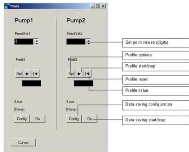
Figure 11-1 PNet pump control software for connection of up to 6 LAMBDA lab instruments
