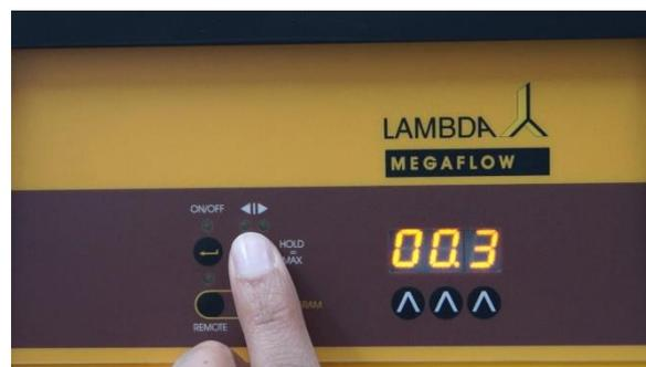
**Figure 2-14** Press  $\triangleleft \triangleright$  button, to set the time resolution.
