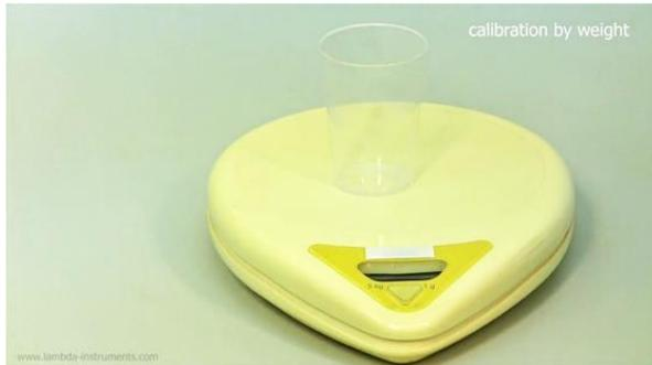
**Figure 3-3** Tare the weighing scale with the measuring beaker (balance with the beaker shows 0.000 g)
