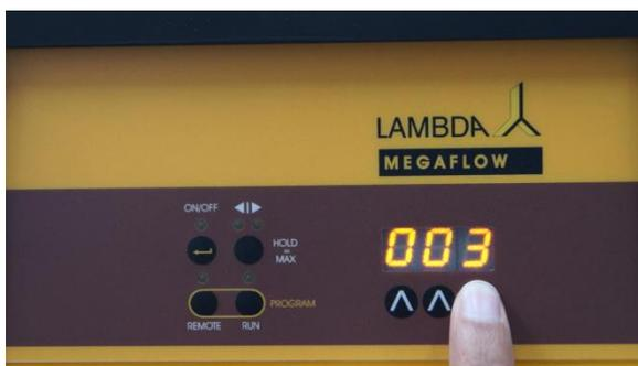
**Figure 2-13** Set the time duration (time) of the second program step.
