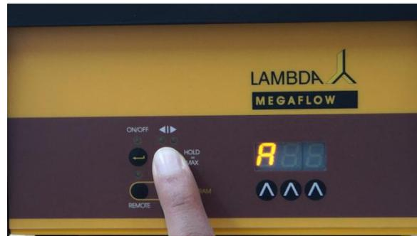
**Figure 4-4** The display of the pump shows message “A” and two numbers. The number from 00 to 99 is the current address of the peristaltic pump.
