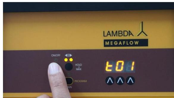
**Figure 2-6** Press the **ON/OFF** button. The indication “t01” will appear for a few seconds on the display indicating that the time period of the first step in minutes, can be entered.
