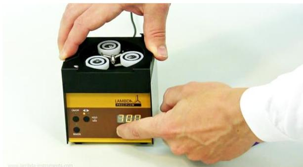
**Figure 1-4** To insert the tubing, the speed of pump can be increased to approx. 700 using the “▲▲▲” arrows present below the LED display. (The tubing can be inserted in the speed range of 300 to 700. In the MEGAFLOW pump, use the lowest speed range for pump tubing insertion).
