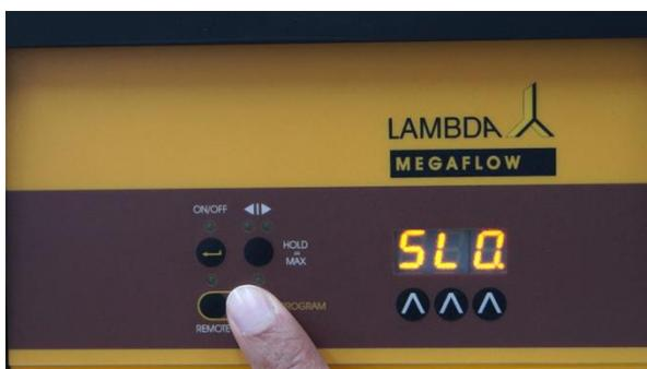
**Figure 1-19** Press the **RUN** button, to select the desired speed mode (**FAS / SLO.**).
