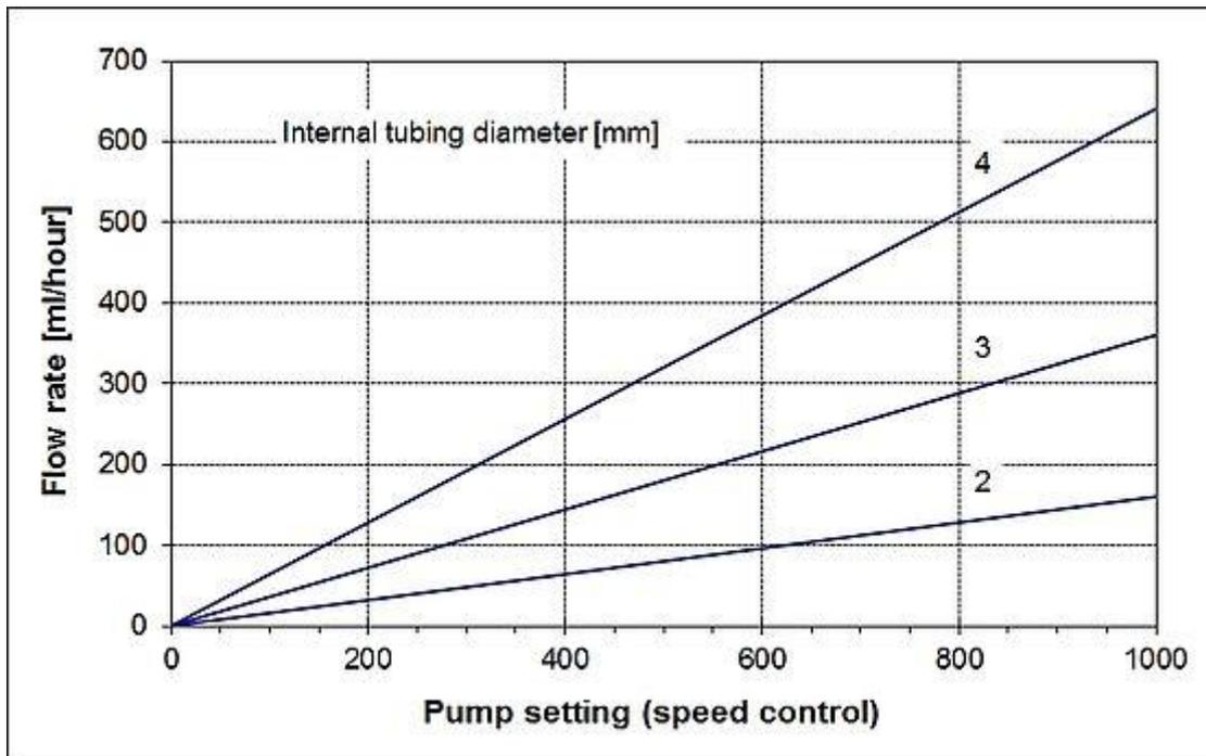
Figure 8-1 PRECIFLOW & MULTIFLOW flow diagram for silicone tubing with inner diameter of 2 mm, 3 mm, 4 mm
