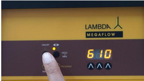
**Figure 1-11** Press ON/OFF button to switch ON the peristaltic pump.
