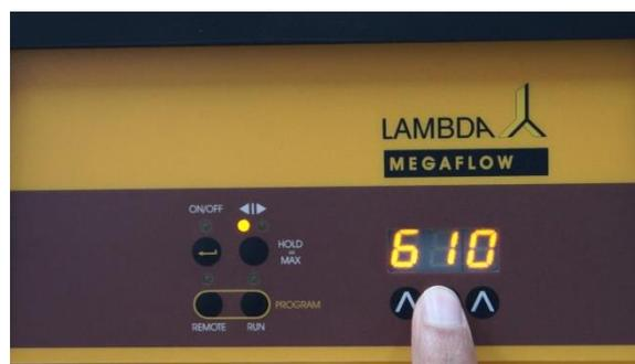
**Figure 1-14** Each  $\wedge$  arrow key changes the corresponding digit on the pump speed above it.
