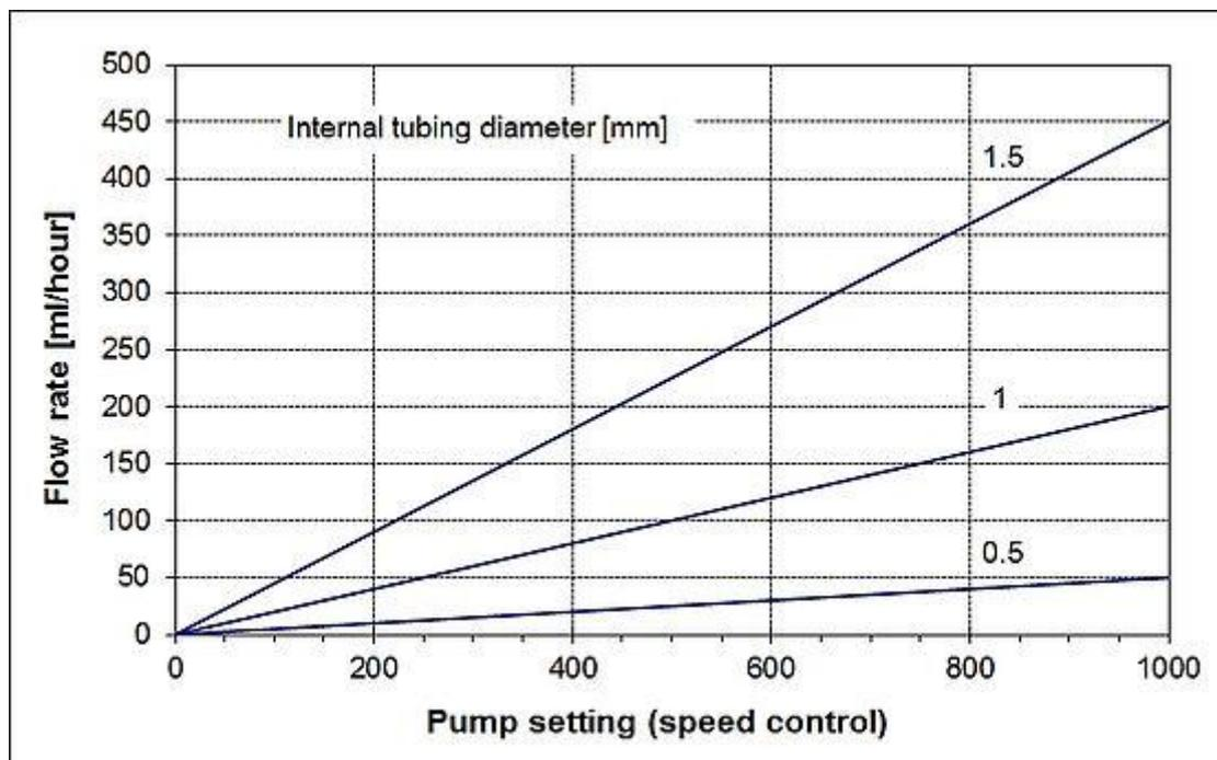
Figure 8-4 Flow diagram of the LAMBDA HiFLOW peristaltic pump when using silicone tubing with inner diameter of 1.5 mm, 1.0 mm, 0.5 mm.
