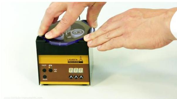
**Figure 1-3** Turn the transparent PVC cover on the pump head either clockwise or anti-clockwise direction to remove it.
