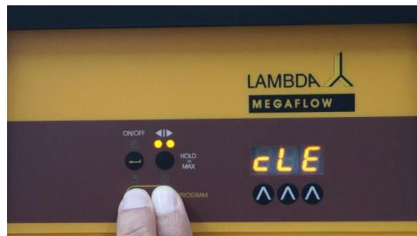
**Figure 2-2** Continuous pressing of **REMOTE** and **RUN** button even after the indication of “PGM” ends up with “cLE” (memory cleared).
