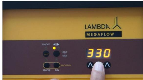
**Figure 2-4** Set the desired speed for the first program step by pressing the buttons  $\wedge \wedge \wedge$  below the display (speed 0 to 999, corresponding to 0 to 100% of motor rotation).
