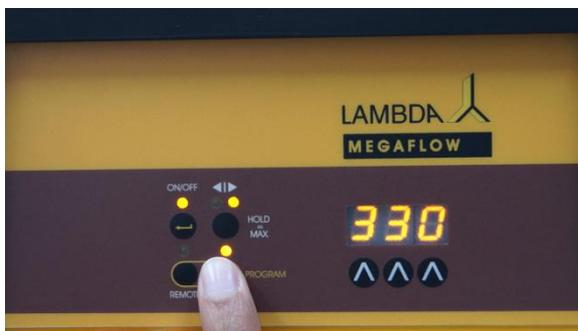
**Figure 2-20** To start the program, press the **RUN** button. The RUN and ON/OFF LEDs are ON.
