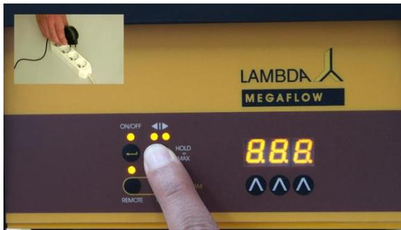
**Figure 4-3** Disconnect the pump from the mains. Keep pressing the direction button ◀▶ and reconnect the pump to power supply.
