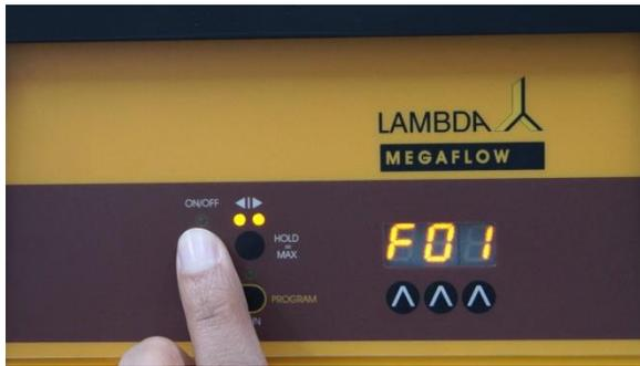
**Figure 2-3** Press the **ON/OFF** button. “F01” appears briefly on the display indicating that the first flow rate value (speed) of the program can be entered.
