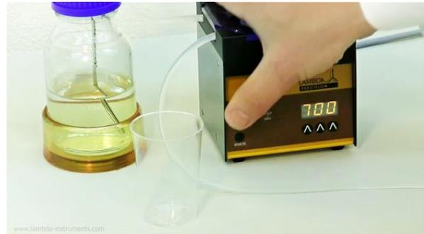
**Figure 3-4** Start pumping of liquid by pressing **ON/OFF** button (PRECIFLOW pump) or **RUN** button to start the program of programmable peristaltic pump (MULTIFLOW, HIFLOW, MAXIFLOW and MEGAFLOW pumps).
