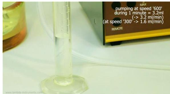
**Figure 3-2** Example: At a pump speed of 600, 3.2 ml of liquid was pumped per 60 seconds. At speed 600, the pump thus achieves a flow rate of 3.2 ml/min. With a **rule of three**, the pump flow rate for other pumping speeds can be calculated.
