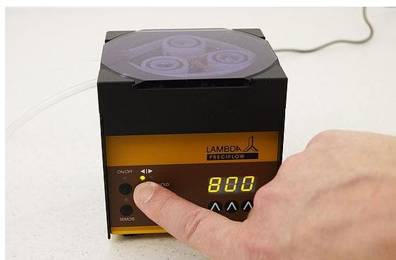
**Figure 1-15** LED illumination in the direction  $\blacktriangleleft$  indicates the clockwise rotation.
