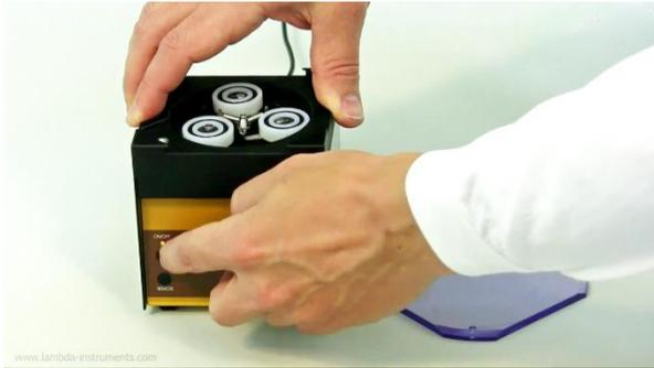
**Figure 1-5** Press the ON/OFF button and select the sense of rotation of the peristaltic pump by pressing the button ◀|▶.
