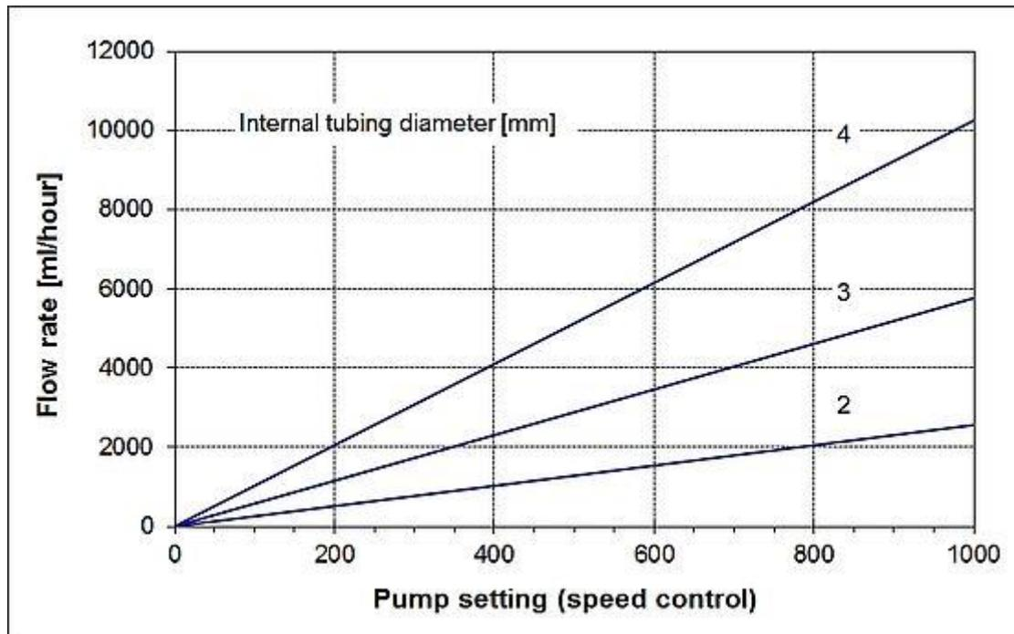
Figure 8-5 Flow diagram of the LAMBDA MAXIFLOW peristaltic pump when using silicone tubing with inner diameter of 2 mm, 3 mm, 4 mm
