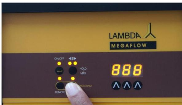
**Figure 1-17** To change the speed mode, connect the power supply of the MEGAFLOW pump and simultaneously press the **RUN** button on the pump control panel.
