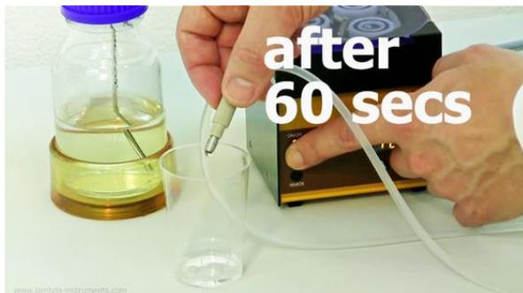
**Figure 3-5** The pumped liquid is collected in the beaker (previously tared in the balance) for a measured time or pre-programmed time (60 seconds).
