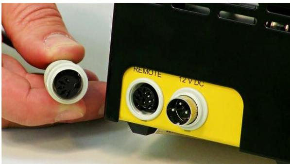
**Figure 1-1** Plug the connector of the power supply into the corresponding socket (12 V DC) at the rear of the peristaltic pump and secure it.
