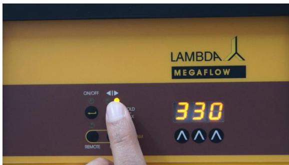
**Figure 2-5** Use the direction button  $\blacktriangleleft \blacktriangleright$  to select direction of flow (clockwise/counter-clockwise).
