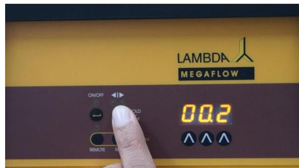
**Figure 2-8** By pressing the  $\blacktriangleleft \blacktriangleright$  button, the time resolution can be set in minutes or 0.1 minutes. In the 0.1 minute time resolution a dot is displayed, e.g. “00.2”. The time resolution can be set individually for each program step.
