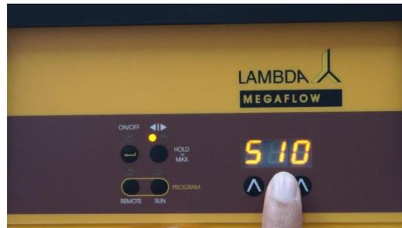
**Figure 2-10** Enter the desired flow rate by pressing the buttons  $\wedge \wedge \wedge$  below the display, for the second program step.
