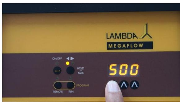
**Figure 1-13** Use the  $\wedge \wedge \wedge$  buttons to set the desired pump speed.
