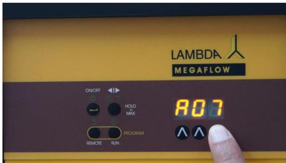
**Figure 4-5** To change the address of the peristaltic pump, press the ▲▲▲ buttons under the display until the desired number is displayed.
