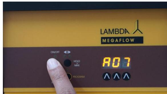
**Figure 4-6** To save the selected pump address, press the ON/OFF button on the peristaltic pump
