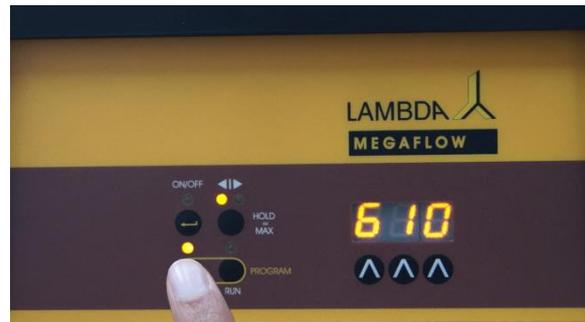
**Figure 4-2** Press the REMOTE button on pump control panel. The corresponding LED lights up and the display indicates the approximate pump speed of the voltage of the external signal.
