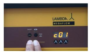
**Figure 2-17** Press the **Remote** and **Run** button simultaneously and you will see the indication "**c01**" on the display. This indicates that the program will be executed only once and the peristaltic pump will stop afterwards.
