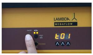
**Figure 2-6** Press the **ON/OFF** button. The indication "**t01**" will appear for a few seconds on the display indicating that the time period of the first step in minutes, can be programmed.
