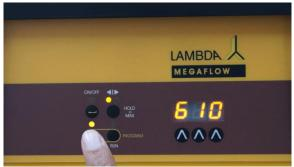
**Figure 4-2** Press the button REMOTE on the front panel. The corresponding LED diode will go on and the display will indicate the approximate voltage of the external signal.
