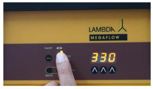
**Figure 1-6** LED illumination in the direction I▶ represents the anticlockwise rotation.
