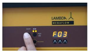
**Figure 2-15** After having entered the time of the last step, press the **ON/OFF** button.
