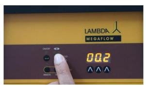
**Figure 2-8** By pressing the **◄I**▶ button, the time resolution can be set in minutes or 0.1 minutes. In the 0.1 minute time resolution a dot is displayed, e.g. "00.2". The time resolution can be set individually for each program step.
