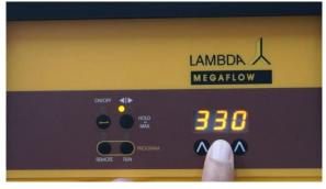
**Figure 2-4** Set the desired flow rate value for the first program step by pressing the buttons **ΛΛΛ** below the display (from 0 to 999, corresponding to 0 to 100% of the motor rotation speed).
