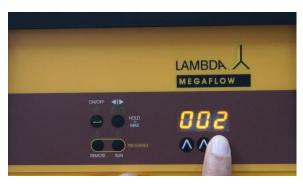
**Figure 2-7** Select the desired time period for the first program step by pressing the buttons  $\Lambda\Lambda\Lambda$  below the display (from 0 to 999 minutes or 00.0 to 99.9 minutes).
