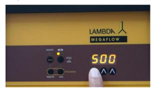
**Figure 1-3** The  $\Lambda$   $\Lambda$   $\Lambda$  buttons can be used to set the desired flow rate.
