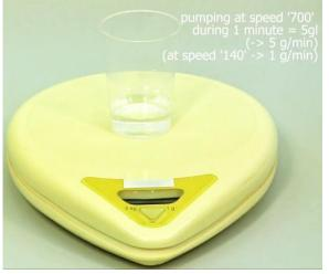
**Figure 3-6** Weigh the measuring beaker with the liquid been collected in the past 60 seconds.
