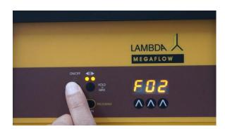
**Figure 2-9** Press the **ON/OFF** button. The indication "F02" will briefly appear on the display.
