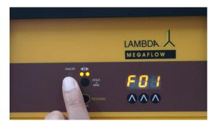
**Figure 2-3** Press the **ON/OFF** button. The indication "**F01**" will appear for a short time on the display indicating that you can select the first flow rate (speed setting) value.
