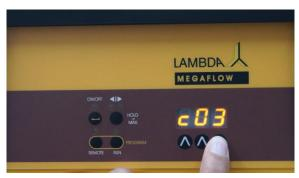
**Figure 2-18** If you wish to repeat the same program 3 times, increase the cycle number to "c03" by pressing the buttons  $\Lambda$   $\Lambda$   $\Lambda$  below the display (from 0 to 99 cycles).
