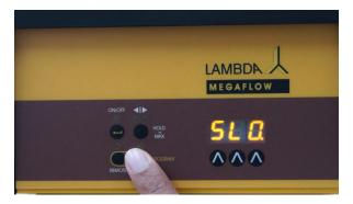
**Figure 1-9** Press the **RUN** button, to select the desired speed mode (**FAS** / **SLO**).
