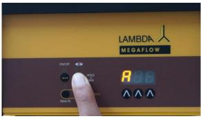
**Figure 4-4** The message "A" and two numbers will appear on the display. This number from 00 to 99 is the current address of the pump.
