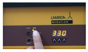
**Figure 1-5** LED illumination in the direction ◀| represents the clockwise rotation.
