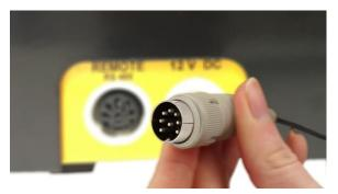
**Figure 4-1** For remote control, connect the 8-poles Pump remote control cable into the 'Remote' socket at the rear of the Peristaltic Pump.
