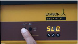
**Figure 1-10** Confirm and save the chosen speed mode by pressing the **ON/OFF** button on the control panel.
