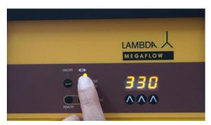
**Figure 2-5** Select the direction of the pump rotation using the direction button ◀I▶.
