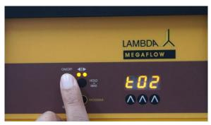
**Figure 2-12** Press the **ON/OFF** button again, the symbol "t02" will briefly appear on the display.
