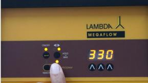
**Figure 2-20** To start the program, press the **RUN** button. The RUN and ON/OFF LEDs are on
