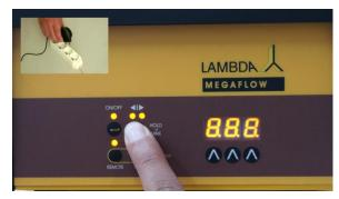
**Figure 4-3** Disconnect the pump from the mains. While keeping the direction button ◀I▶ pressed, connect the pump to the mains again.
