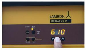
**Figure 1-4** Each  $\Lambda \Lambda \Lambda$  arrow can be used to change the corresponding digit on the flow rate.
