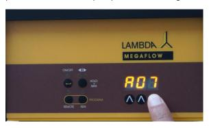
**Figure 4-5** To change the address press the buttons  $\Lambda$   $\Lambda$   $\Lambda$  under the display until the desired number is obtained.
