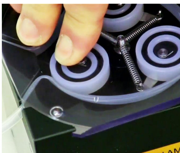
Figure 1-10 Turn the cover so that the steel ball embedded in the left-front corner of the peristaltic pump fits into the notch in the cover.
