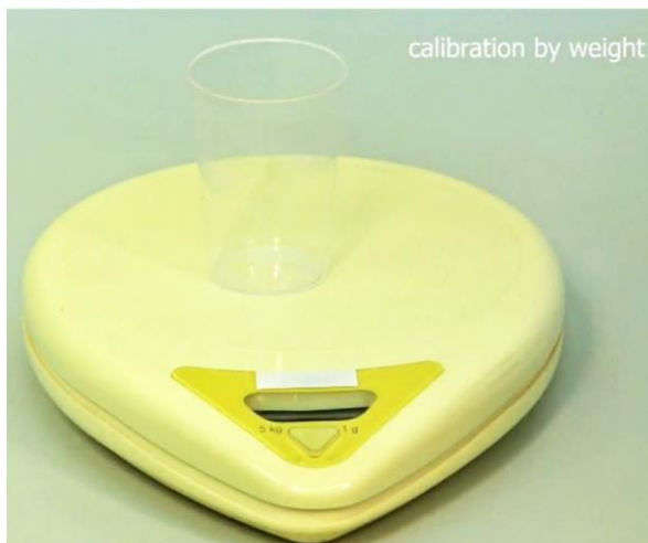
Figure 3-3 Measure the weight of the empty beaker using a sensitive weighing scale. For the exact measurement of the liquid collected, tare the weighing scale with the measuring beaker (Example: 0.000 g).
