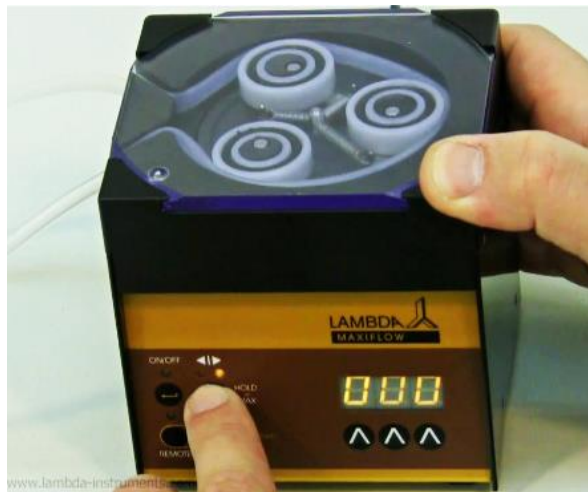
Figure 2-4 Select the direction of the pump rotation using the direction button ◀▶.
