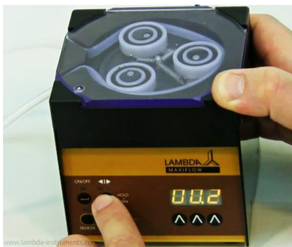
Figure 2-8 By pressing the ◀▶ button, the time resolution can be set in minutes or 0.1 minutes. In the 0.1 minute time resolution a dot is displayed, e.g. “00.1” . The time resolution can be set individually for each program step.
