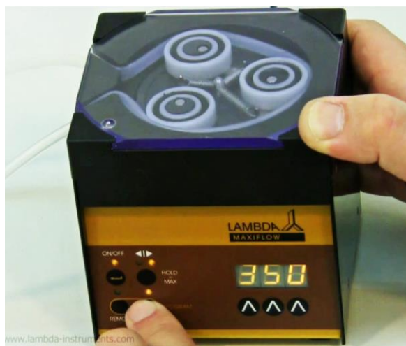
Figure 2-20 To start the program, press the RUN button. The RUN and ON/OFF LEDs are on.
