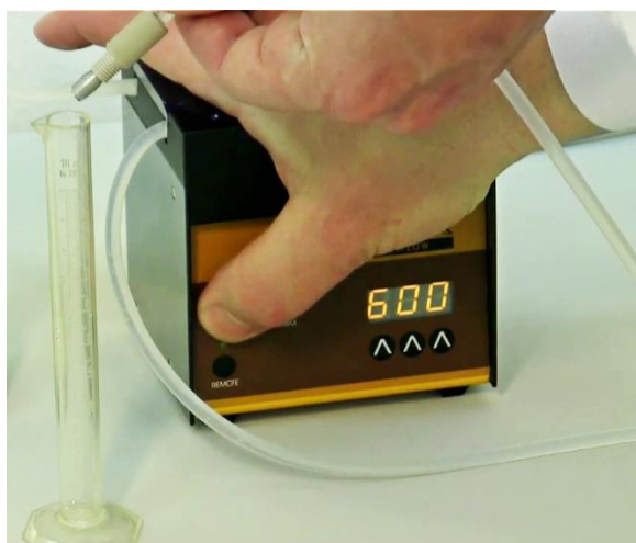
Figure 3-1 Turn on the pump and have the other end of the tubing ready near the measuring cylinder. Carefully collect the liquid being pumped in the measuring cylinder for about 60 seconds.
