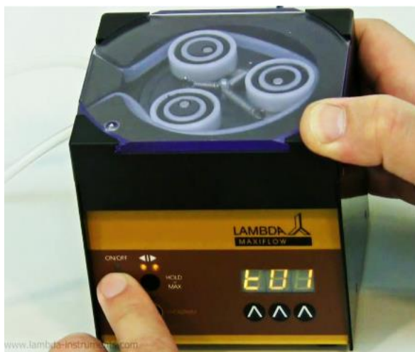
Figure 2-6 Press the ON/OFF button. The indication “t01” will appear for a few seconds on the display indicating that you can program the time period of the first step in minutes.
