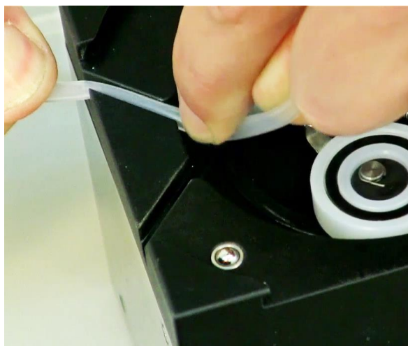
Figure 1-6 Press the tubing into the back slot on the top of the peristaltic pump. Thin tubing should be pushed completely to the bottom.
