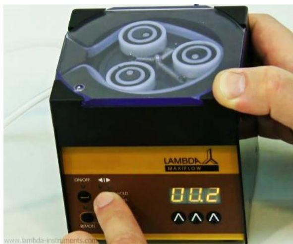
Figure 2-14 Press ◀▶ button, to set the time resolution.
