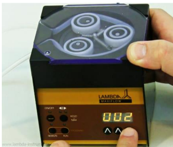
Figure 2-7 Select the desired time period for the first program step by pressing the buttons ▲▲▲ below the display (from 0 to 999 minutes or 00.0 to 99.9 minutes).
