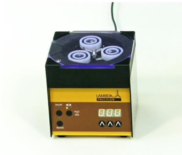
Figure 1-2 Plug the power supply into the AC mains (90-264V/50-60 Hz). After a short beep signal, the display will be illuminated. The last used settings will be displayed.
