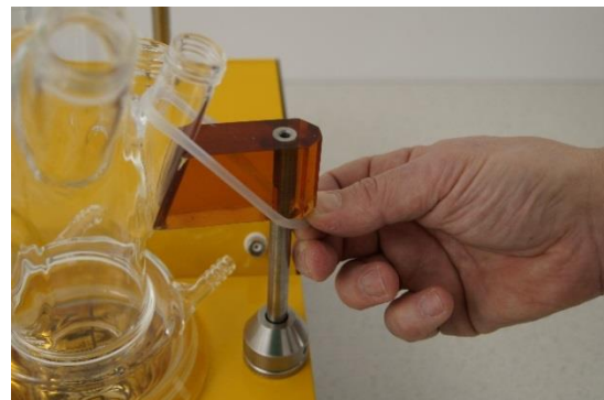
Figure 7 Elastic silicone ring helps to affix the vessel to the adjustable lateral holder
