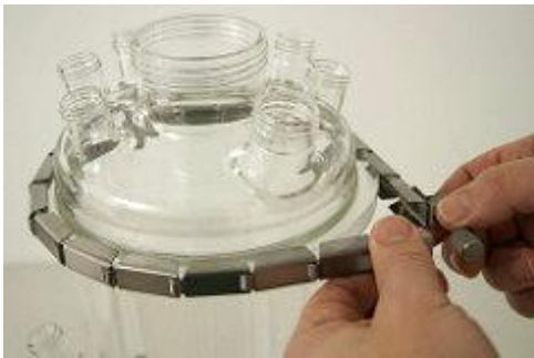
Figure 13 Installation of 7 L culture vessel
